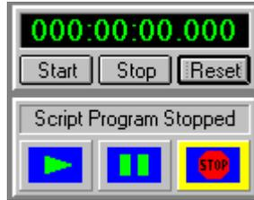
The panel indicates the current status of the script program, along with three buttons that can be used to start, pause, or stop the script program execution.
